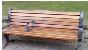
Park bench with two armrest for persons who need assistance on both sides when wanting to get up.
